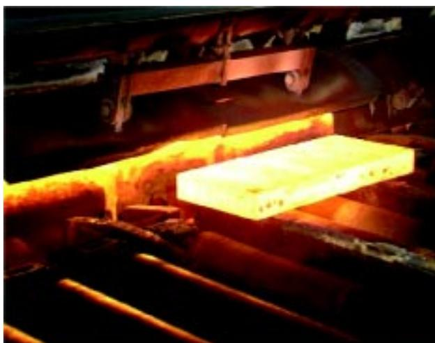
*A slab emerging from a furnace.*
