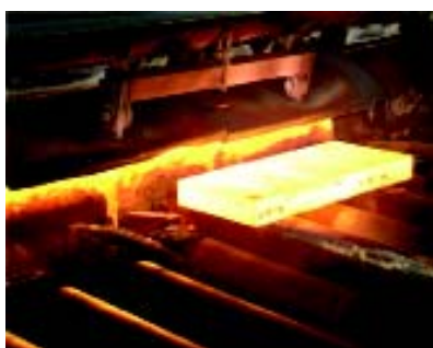
A steel slab exiting a re-heating furnace where the slab is heated up to 1200°C. The position of the slab and the measurements from the heating environment are tracked and a prediction for the exit temperature of the slab is given using the software developed in the VALTA and TASA data mining projects.
