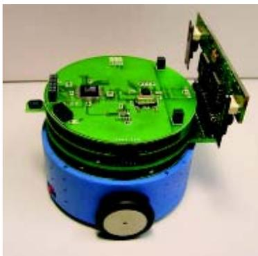
*The miniature mobile robot developed in the Computer Engineering Laboratory of the University of Oulu. The modules shown here are (from the top): the radio, the environment, and the stereo camera modules, respectively. All modules have an 8-bit low power 8MHz MCU (ATmega32), which implements the serial interface for accessing the module services, and controls the logic in the module.*
