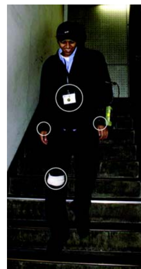
User activity measurement with wearable 3D acceleration sensors (on the right wrist and thigh, triaxial accelation signals).
