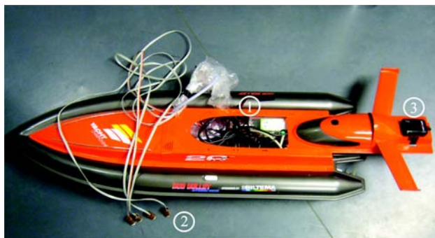
A prototype of a robot boat for sensing aquatic environments: 1) an embedded computer with a WLAN communication interface, 2) sensors, and 3) GPS positioning system.
