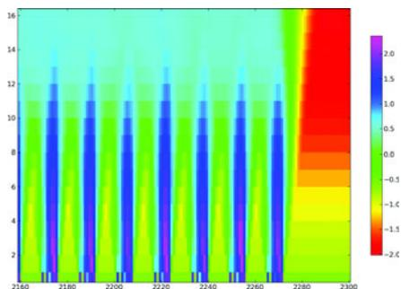
Visualization of entropy in a OpenVPN keyfile. Field borders can easily be seen.
