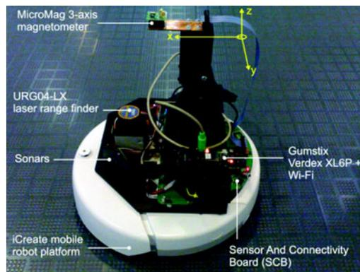
Top left: a geometrically distorted map (from the CSE laboratory) based on odometric data only. Top right: a geometrically consistent map provided by the SLAM technique that is based on the utilization of the ambient magnetic field. Bottom: the robot used in the real-world experiments.
