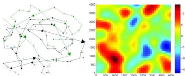
Left: particle distribution after 40th iteration on a sine mean function. The black and green arrows are the true and mean control (odometry) paths, respectively. The grey dots represent particles, red dots expected sensing sites and blue dots are the most likely sensing sites. Right: an illustration of a component of the true vector field used in the simulations to emulate the ambient magnetic field, which provides the necessary information for the proposed nearoptimal SLAM.
