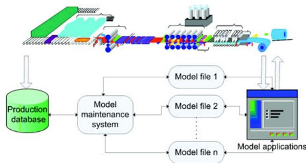
The model maintenance system processes production data to keep up-to-date the prediction models used by software applications whose purpose is to improve production efficiency.
