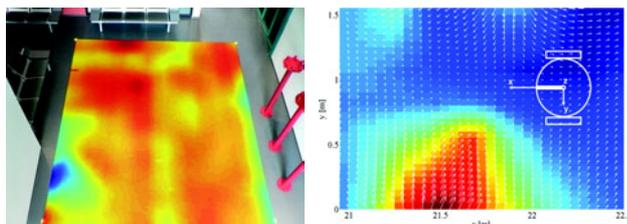
An indoor ambient magnetic field (left) and a close up from an ambient magnetic field showing the magnitude of the field (color) and the direction of the field (arrows) in  $x$ - $y$  plane.
