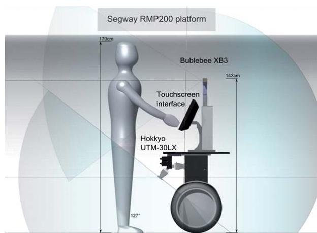
Figure 5. A test setup for the Human-Robot Interaction.
