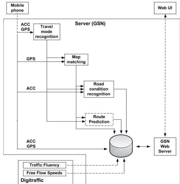
Figure 4. An SDFA prototype collecting data with mobile phones attached to vehicles and analyzing road conditions from the collected data.
