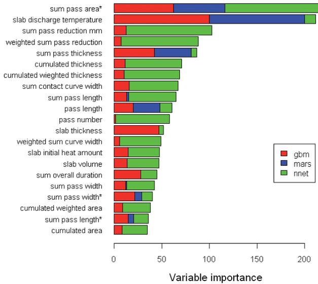
A variable importance plot on the variables most valuable in the prediction of rolling temperatures.
