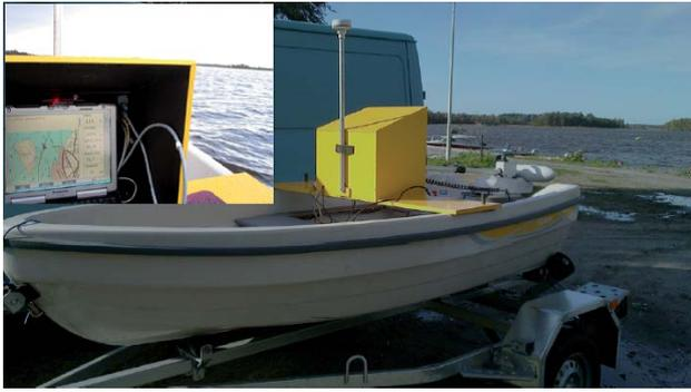
The USV developed in CSE. The USV can be used as an autonomous measurement instrument in aquatic environments. Top left: the USV is performing a measurement mission in the Baltic Sea, Pietarsaari, Finland.
