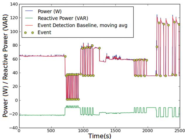
Detection of appliances on-off events from single point measurements. Furthermore, typical power “finger prints” in the feature space to be used to discriminate between different devices in the load monitoring system are visualized.
