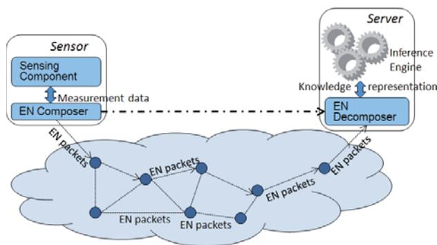
*Resource-constrained sensors and an inference engine communicate by exchanging EN packets.*
