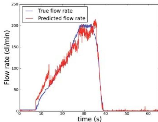
A water flow estimation system based on the mechanical vibration of the water pipe and statistical learning methods.
