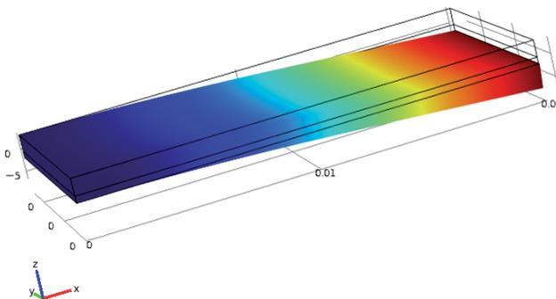
The cantilever beam structure was optimized to produce a maximal displacement at a 4000 Hz resonance frequency. The amount of displacement is indicated with the colour ranging from blue to red.
