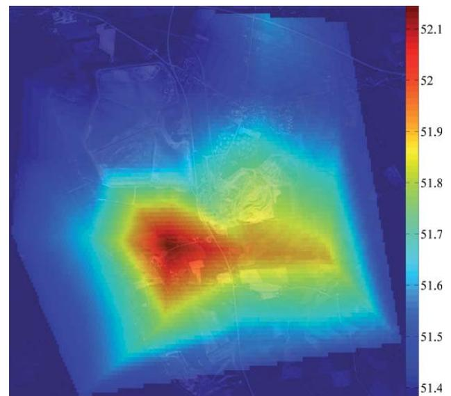
The aeromagnetic map [ $\mu\text{T}$ ] of the Pyhäsalmi mining area superimposed with an aerial photo. The aeromagnetic data is collected from an altitude of 150 m. The magnetic field of the mining area has a unique spatial pattern which stands out from the background magnetic field. This is a typical phenomenon in areas where magnetic minerals (e.g. iron ore) can be found.
