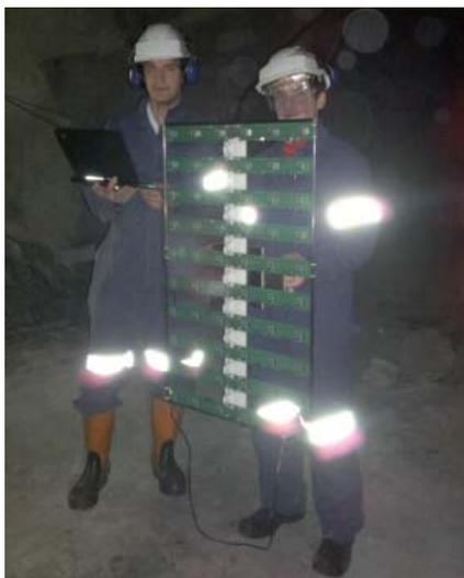
The magnetometer array used to collect the magnetic field data. The magnetic field maps used in the experiments were generated using the measurements performed by one horizontal row of the sensor array. The photo has been taken on level 2 of the Pyhäsalmi mine, 1440 m below the surface.
