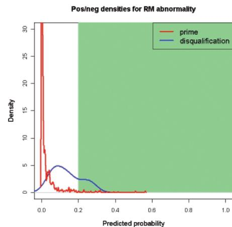
The density functions of the predicted disqualification probability calculated from the composition and planned production method for products that are finally qualified or disqualified in the qualification test.
