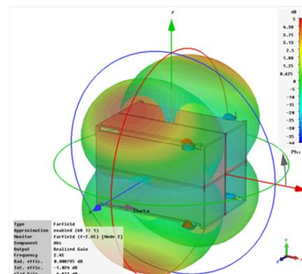
Figure 2. Example of antenna radiating pattern from [Sonkki et al., "Four slot MIMO cube ...", XXIX URSI National Symposium, Valencia, Spain].
