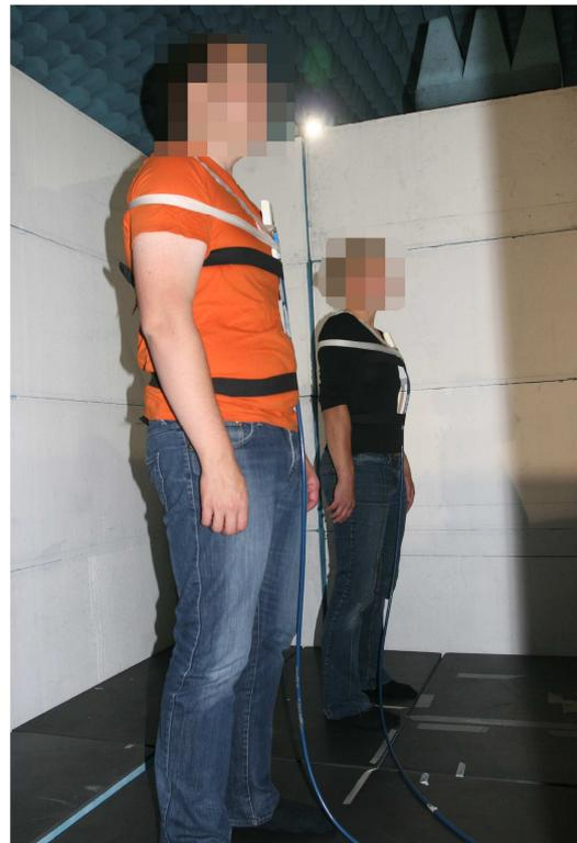
Figure 4. Body area network measurement.
