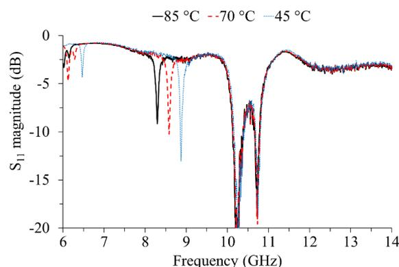
Effect of interconnection cracks on RF performance of an antenna assembly during shifting temperatures [J. Putaala et al., (2011), IEEE Trans. Compon. Packag. Manuf. Technol. 1:1465].
