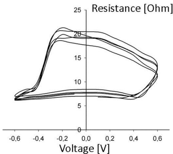
Current-voltage response of a memristor [M. Nelo et al., (2013), Japanese Journal of Applied Physics 52(5): article 05DB21].
