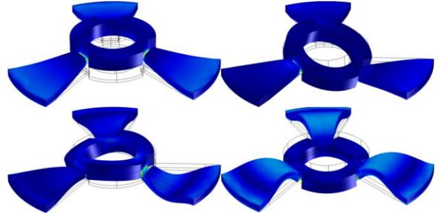
Different resonance modes for FPI-actuator [M. Sobocinski et al., (2012), IEEE trans. on Ultrasonics, Ferroelectrics and frequency control 59(9): 1990–1995].
