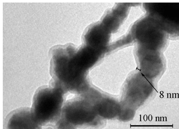
*Transmission electron microscopy image of metallic cobalt nanoparticles coated with an 8 nm thick layer of fatty acid surfactant. Utilization of surfactant layer enabled formulation of stable inks from the dry nanoparticle powders [M. Nelo et al., (2010), Progress In Electromagnetics Research 110: 253–266].*
