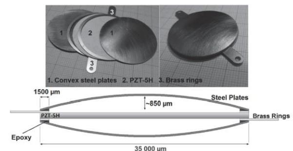
The cymbal structure and the individual parts of the shoe mounted piezoelectric harvester [M. Leinonen et al., (2014), Journal of Intelligent Material Systems and Structures, 25(4):391–400].
