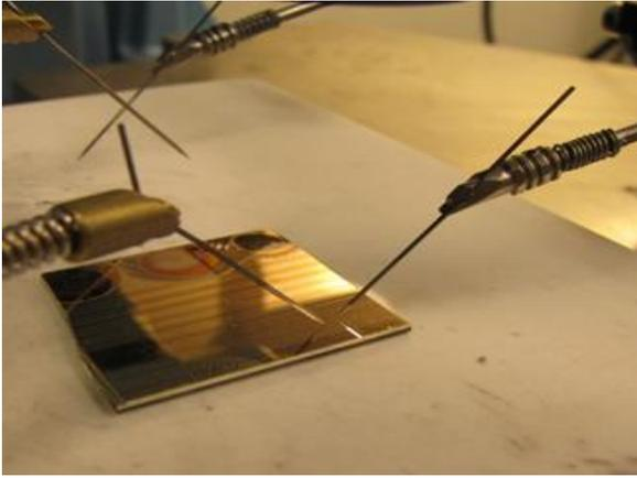
Measurement being done to inkjet-printed memristive pattern.
