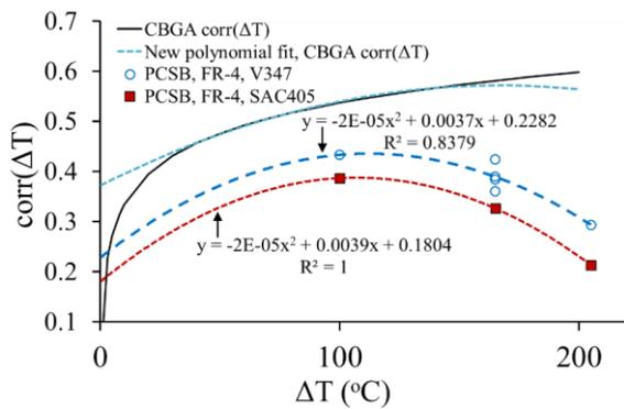
Temperature range dependency of correction terms in modified Engelmaier's model for BGA interconnections [J. Putaala et al., (2012), IEEE Trans. Compon. Packag. Manuf. Technol. 2:994].
