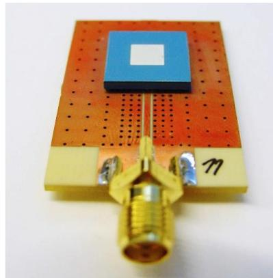
Ceramic patch antenna module (blue) attached on an RF printed wiring board using PCSB BGA interconnections [J. Putaala et al., (2011), IEEE Trans. Compon. Packag. Manuf. Technol. 1:1465].
