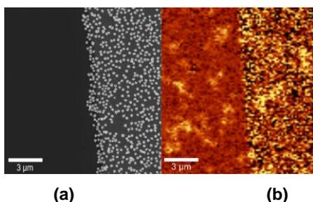
Figure 8. SEM image of the gold nanoparticle layers onto conventional waveguides (a); image of the intensity of Raman signal.
