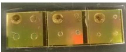
Figure 6. PDMS chambers on top of SERS polymer Klarite surface for concentration and even drying of *L.innocua* samples.
