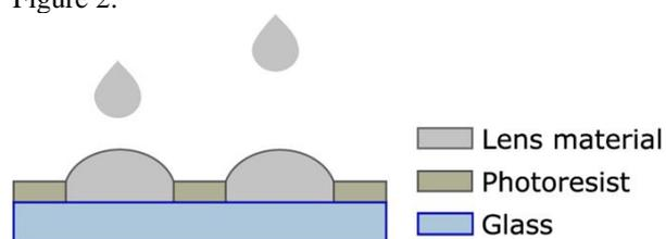
Figure 1. The lenses are printed onto the patterned substrate drop by drop, until the shape is at wanted curvature.
