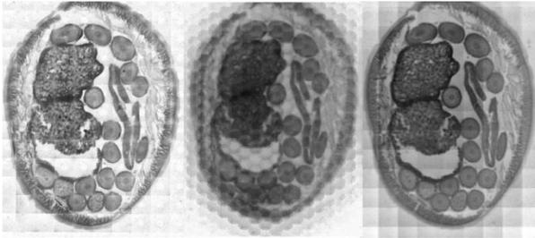
Figure 3. Comparison of images made with different lens arrays. From left to right: glass lenses, hot embossed polycarbonate lenses and the proposed inkjet printed lenses. The polycarbonate lens array produces the lowest image quality. The inkjet lenses produce images with quality comparable to the class lenses.
