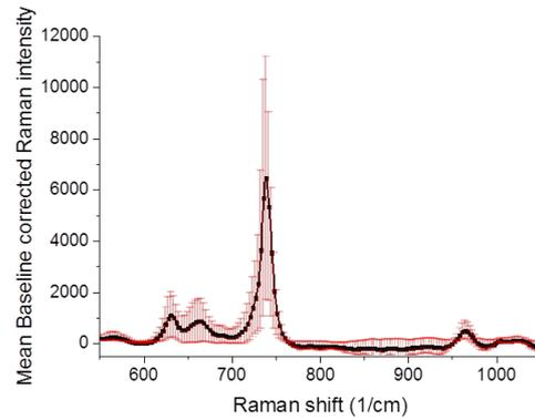
Figure 4. Raman spectrum and mean absolute deviation of a  $6.8 \times 10^9$  cfu/ml *L.innocua* sample droplet on polymer Klarite with nanoparticle enhancement.
