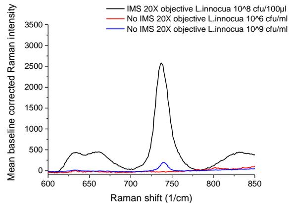
Figure 5. Raman spectra of *L.innocua* sample droplets on polymer Klarite with and without immunomagnetic separation beads.
