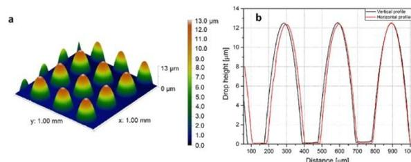
Figure 2. (a) 3D-profile of the printed MLA. (b) Graphs of the vertical and horizontal profiles of the MLA. The average height and diameter of the lenses is 12.4  $\mu\text{m}$  with standard deviation of 0.06  $\mu\text{m}$  and 222  $\mu\text{m}$  with standard deviation of 4.61  $\mu\text{m}$ , respectively.
